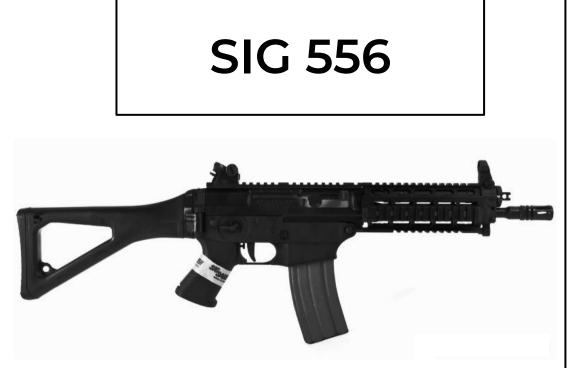
The Sig 556 is a shorter and lighter variant of the Sig 550 assault rifle. The Sig 556 is a 5.56 ×45mm NATO, air-cooled, gas piston, magazine-fed carbine. It has a 10.5 inch barrel and a telescoping stock. This short barrel, fully automatic version was used by SWAT teams across the US.
