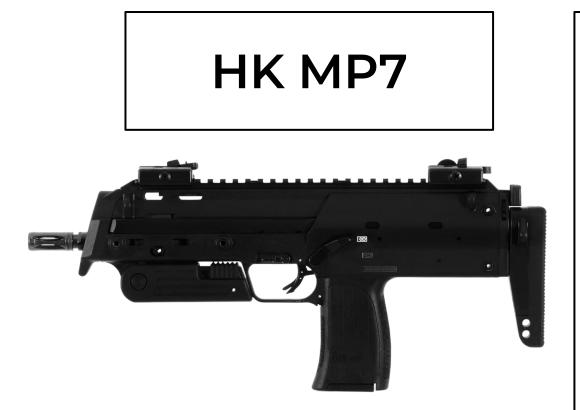
The MP7 is the newest submachine gun designed by Heckler & Koch as a replacement for famous MP5. The MP7 is a closed bolt, gas-piston PDW that fires the armour piercing 4.6x 30 from a detachable box magazine. With a high fire rate and low recoil, it is rapidly becoming a favorite of special forces and police across the globe.
